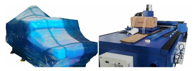
2. Remove the packing materials on the control console, and set it to the front of the left side of the machine.
