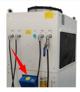
3. Connect the alarm signal to the machine.
