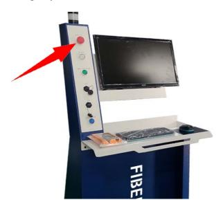
Release the emergency button on 6kW lasers.
