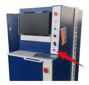
9. (For 3kW only) Turn on the fiber laser.
