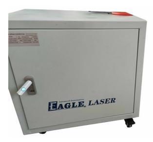
6. Remove the packing materials on the chiller, and set it to the rear of the left side of the machine.
